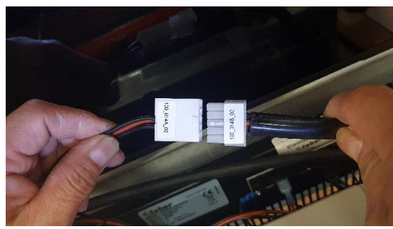
4a. Connect the heat fan cable with the Engine (cable no: 100_014A_02 and 100_014B_02).
