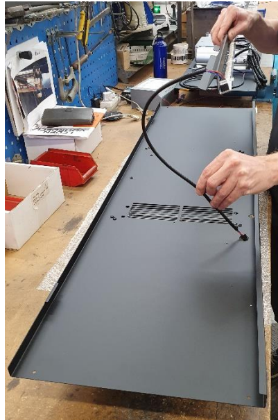
2a. Insert the connection cable through the hole....
