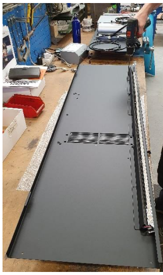
2b. ... and fix the LED support with supplied screws.
