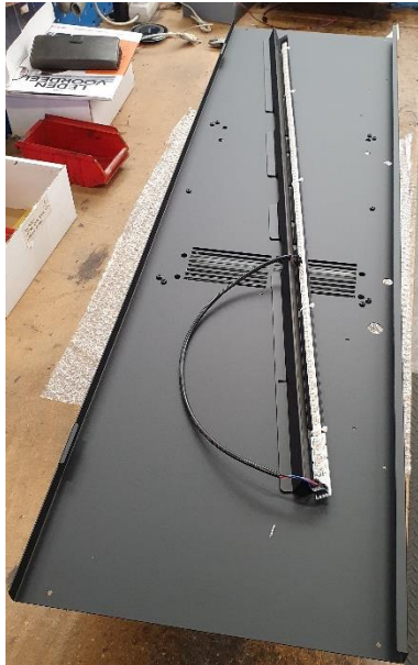
1. Fan/heater unit + top light.
