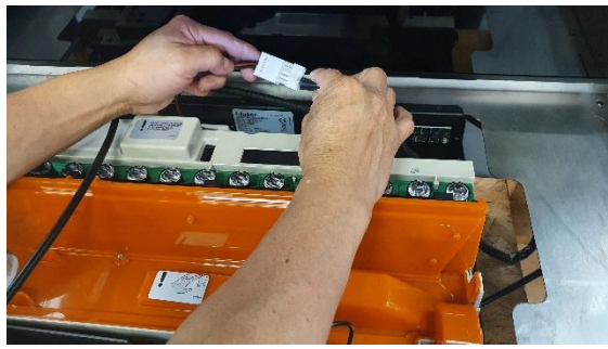
4a. Connect the heat fan cable with the Engine (cable no: 100_014A_02 and 100_014B_02).
