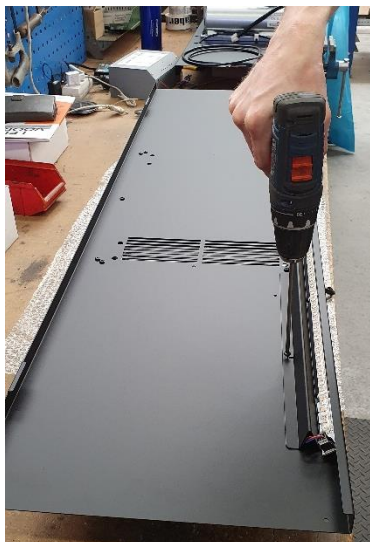
2b. ... and fix the LED support with supplied screws.
